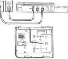
Follow these steps if the station will be installed on screws securely fastened to the wall. If telephone lines 1 and 2 are on one jack and tele phone lines 3 and 4 on another jack see the following connection drawing. Otherwise go to step 13.
